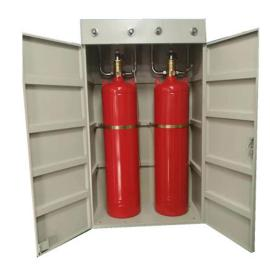
Welded cylinder made of steel, fire extinguishing agent(HFC-227ea, same as FM200), clamp, cabinet, container valve, solenoid actuator, high pressure hose, nozzle and pressure switch. If a cylinder's capacity is 120Ltr or more than 120Ltr, we suggest that each cylinder could be equipped with 2 nozzles and 2 high pressure hoses, in order to make sure the agent can be fully relised according to the discharge time standard.
